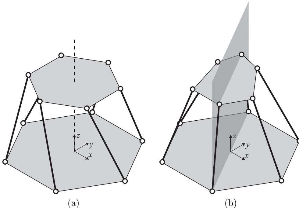
Figure 7: Stewart platforms that are in singular positions due to the presence of symmetry: (a) a Stewart platform with  $C_6$  symmetry about the  $z$ -axis, shown dashed; (b) a Stewart platform with  $C_s$  symmetry in the  $x = -y$  plane, shaded.
