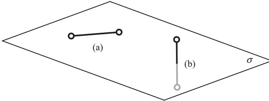
Figure 6: Possible placement of a bar unshifted by a reflection in a plane: (a) lying in the plane; (b) lying perpendicular to the plane.
