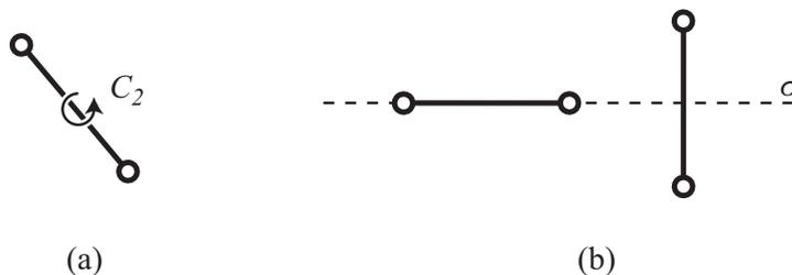
Figure 2: Possible placement of a bar with respect to a symmetry element in two dimensions, such that it is unshifted by the associated symmetry operation: (a)  $C_2$  centre of rotation; (b) mirror line.
