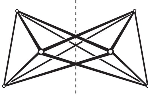
Figure 2: An example of an isostatic framework with reflection symmetry (the mirror plane is indicated by a dotted line). This  $\mathcal{C}_s$ -symmetric framework is non-planar. Larger and smaller circles indicate joints that lie respectively in front of, and behind the median plane of the framework.
