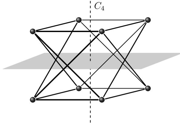
Figure 4: A framework which is symmetry-regular with respect to  $\mathcal{C}_{4h}$ .
