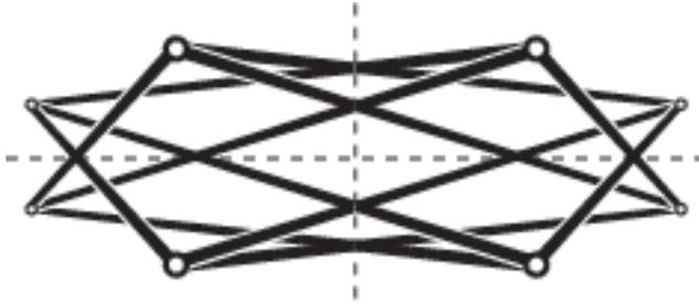
Figure 5: An example of an over-constrained framework with  $\mathcal{C}_{2v}$  symmetry based on a non-planar realisation of the complete bipartite graph  $K_{4,4}$ . As in Fig. 2, dotted lines indicate mirror planes and larger and smaller circles indicate joints that lie respectively in front of, and behind the median plane of the framework.
