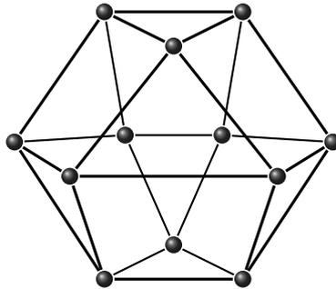
Figure 3: A bar-and-joint framework connected as the skeleton of the cuboctahedron.
