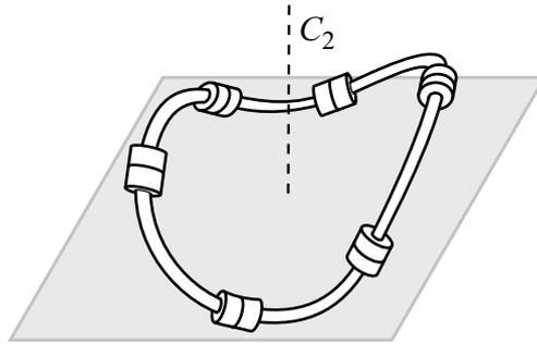
Figure 6: A schematic view of a 6-loop, adapted from Guest and Fowler (2010). Six curved bodies are connected by six in-line revolute joints, each of which allows a single, twisting, degree of freedom.
